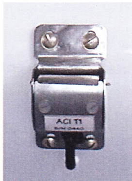
Fig.1- Stall speed vane on the left wing
